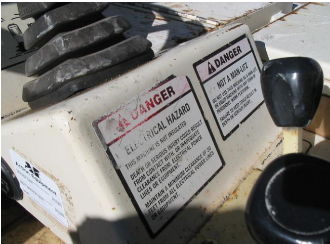
Photo 3 Warning Plate Inside Cab (courtesy of OSHA)
