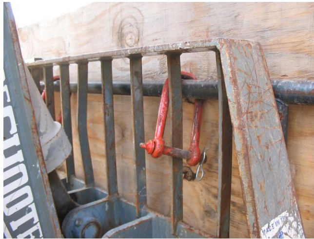
Photo 6 Platform fastened to forks (courtesy of OSHA)
